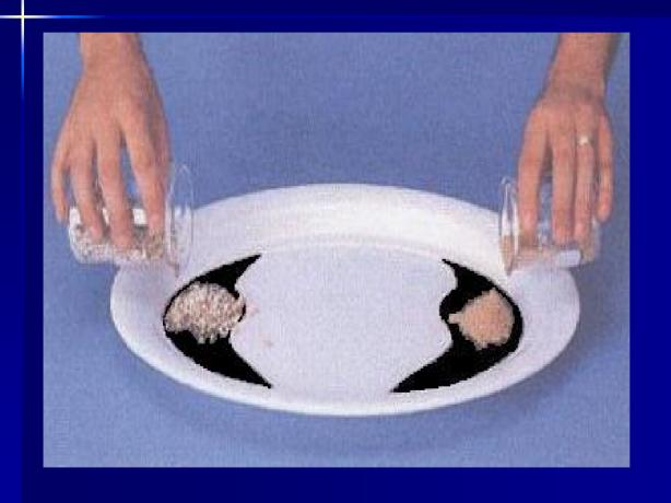
Pour equal portions (by weight) of Floor Gator & Floor Dry on each spill.
