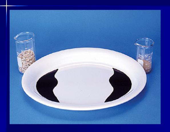
Pour two (2) equal portions of used motor oil onto a clean white plate.
