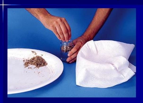
Place used oil & Floor Gator mixture into a glass jar half full of cold water.
