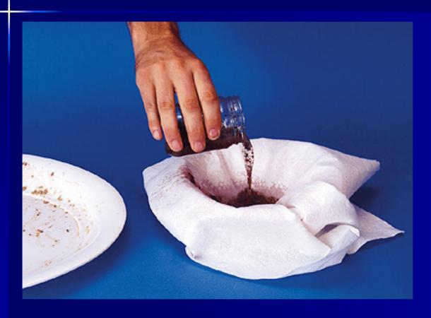
Pour the used oil Floor Gator mixture onto a cotton wipe, coffee filter or paper towel.
